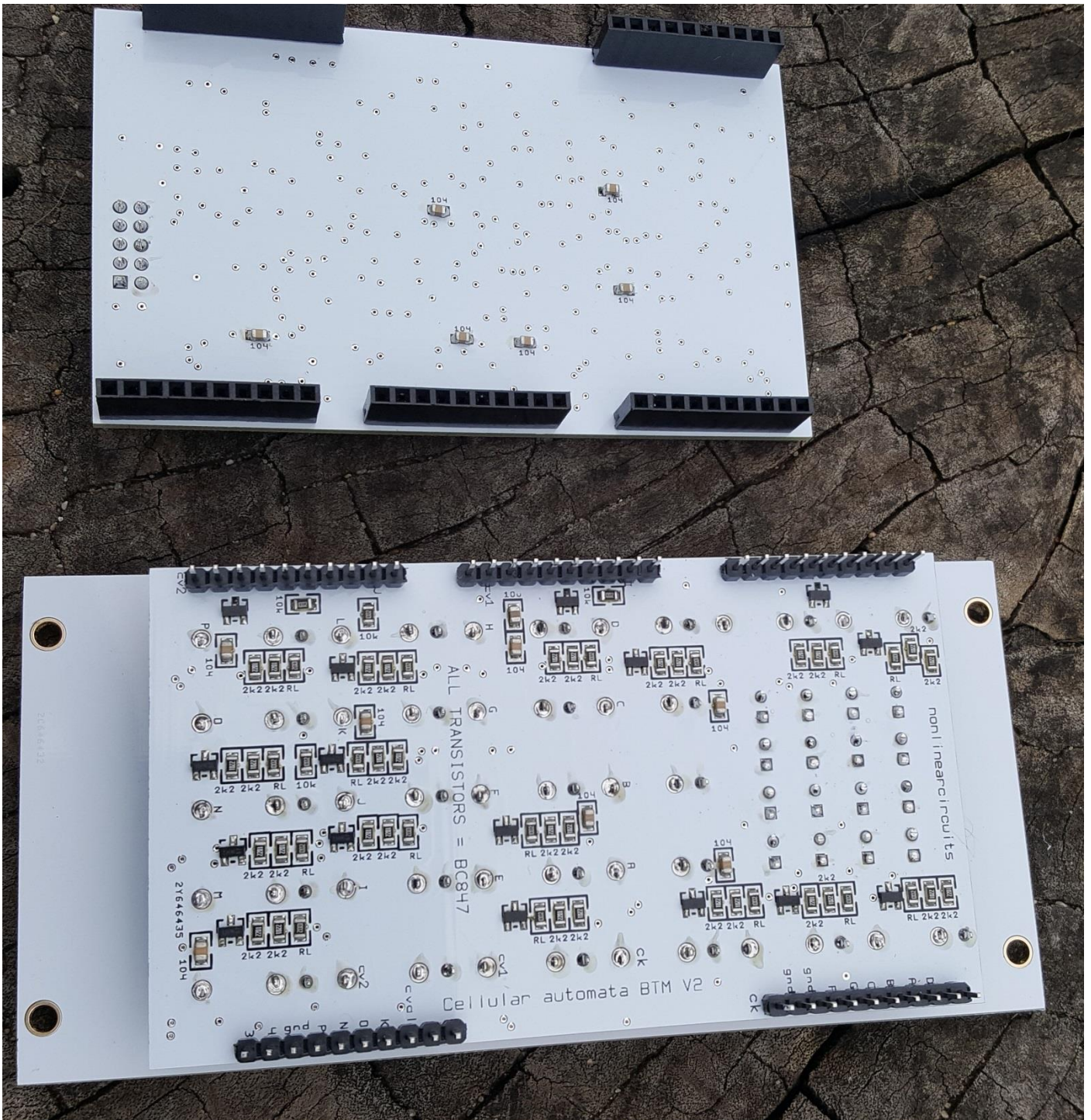
Note - 6 100nF capacitors are placed on the bottom of the upper PCB
